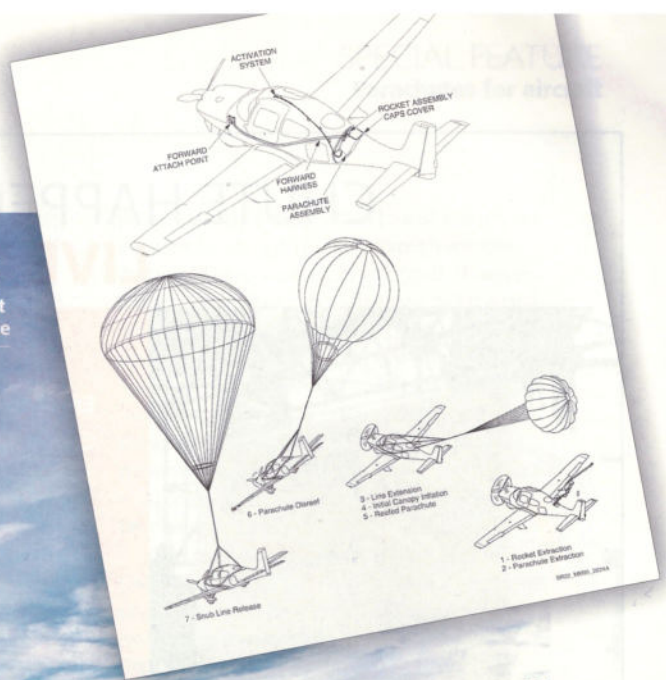
BRS airframe location and deployment sequence
